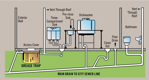
Grease traps capture grease and oil from wastewater flow and store them in a tank under the kitchen floor or near dishwashers.
