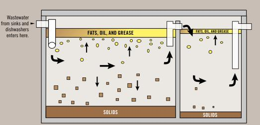
Grease interceptors hold fats, oils, greases and solids in a tank where they settle to the bottom until they can be removed. Grease traps and grease interceptors essentially work the same and both keep fats, oils and grease out of city sewers and the environment.
