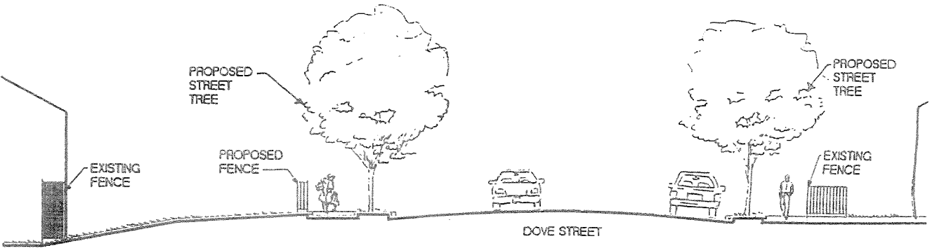
DOVE STREET IMPROVEMENTS CROSS SECTION A-A
